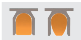
Fig. 1 A patent-protected recess in the milled female parts makes for a perfect fit, prevents spring effects when strongly activated and guarantees durable functioning. As a result, there is a noticeable slight snap action with the resilient bar.
