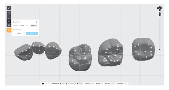
Always check the margin and internal aspect of the restoration to confirm that supports have not been generated in those critical areas. If additional support is needed, manually add supports where appropriate.
