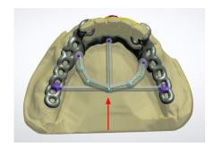
When designing clasps thinner than 0.8 mm, connect the clip arms together for the most accurate results.
