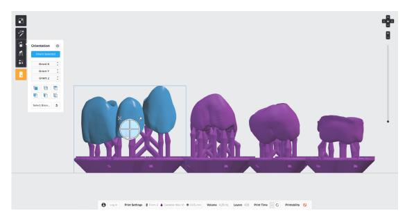
For full contour crown and bridge patterns, place support touchpoints on the cusp tips and ideally not on the contact areas of the crown.
