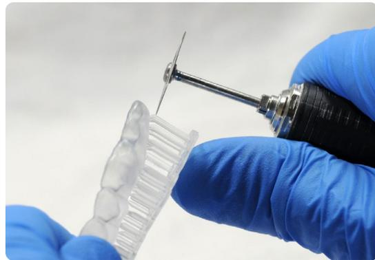
**Note:** While ripping the supports from the part might be quicker, it can leave divots in the part. We recommend cutting the supports off individually.
