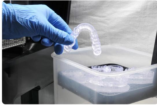
**Note:** Using a squeeze bottle of fresh IPA and compressed air can help make parts clean, especially in deep parts of the intaglio anatomy.
