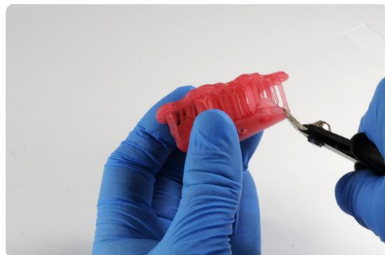
Small, sharp scissors can be used to cut the supports closer to the part as a second step.
