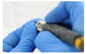
Check printed part fit and finish. Contour parts as needed using a dental handpiece and carbide rotary burs.
