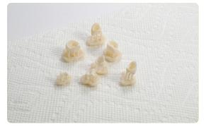
If any wet, uncured resin is still present after drying, use a squeeze bottle with fresh IPA to remove uncured resin and then air dry the parts again.
